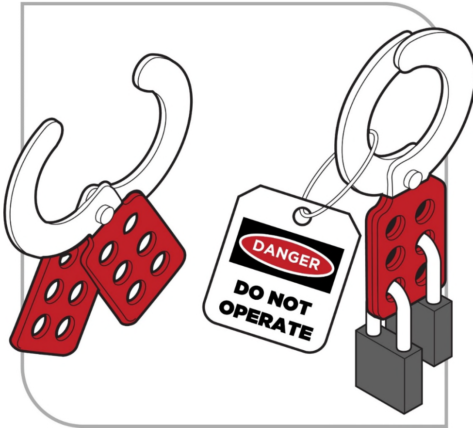
Figure 3 Example of tag and lockout with padlocks
